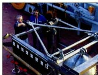
Left: the junction box on deck, showing the submarine connector plug board. Right: Connecting the cable to the junction box.
