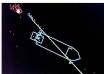
Left: real-time display from the acoustic navigation computer. Castor's position is relative to the cable lay, with the junction box current position (red box) during descent. The red spots are previous junction box positions during the ship's motion. Right: deployment of the linked "triplets" of glass pressure spheres containing photomultiplier tubes on the 60 m test line. (Papillaut/Dars CNRS and Circella INFN Bari.)
