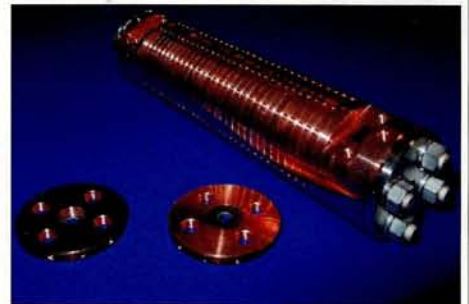
A 30-cell accelerating structure used in the CLIC Test Facility (CTF2), together with a copper cell (left) and a molybdenum insert.
