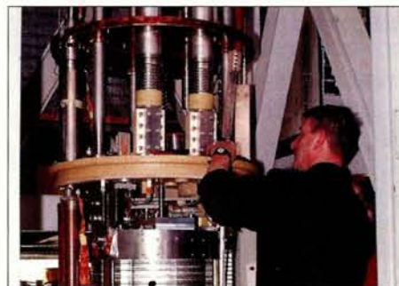
The first matching quadrupole magnet leaves the cryostat after successful testing.
