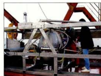
Left: the junction box on deck, showing the submarine connector plug board. Right: Connecting the cable to the junction box.
